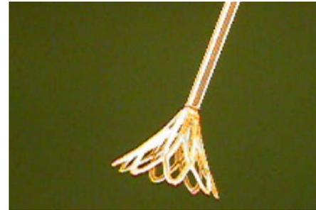
Deformed above  $T_g$ , then cooled to fix secondary shape
